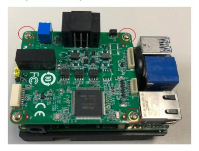
Step 4: Plug in cable with the board.
