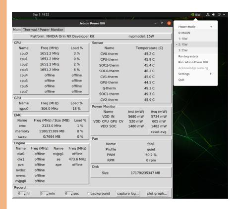
**Note**: Power mode is dependent on DRAM size. For more detailed information please visit: <a href="https://developer.nvidia.com/embedded/jetson-modules">https://developer.nvidia.com/embedded/jetson-modules</a>
