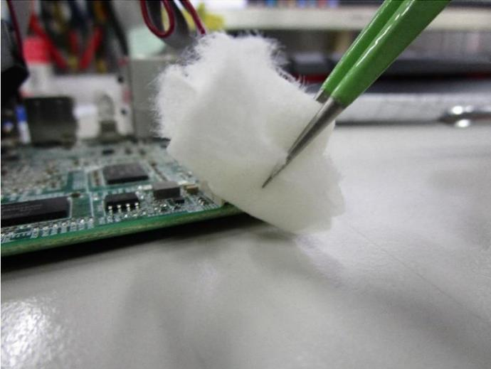
**Step 3:** Let soak for 10 more seconds, then use anti-static tweezers to remove the glue.
