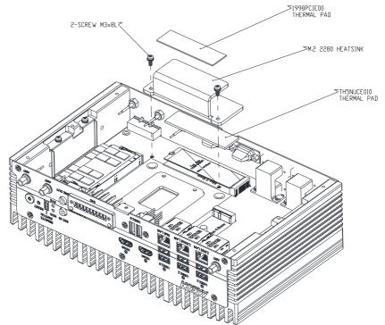
**Step 4**: Prior to reassembling the system bottom cover, ensure a second thermal pad is placed on top of the M.2 2280 Heatsink.
