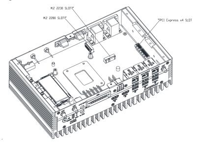
**Step 3:** For M.2 2230 and PCle cards, follow standard installation procedures of inserting each card at a slight angle ( $\sim$ 30°) and gently pressing down until fully seated. Secure the free end of the card(s) with their respective retaining screws.
