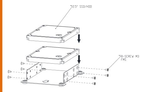
Note: Ensure the SATA connectors face outward for easy cable access later.
