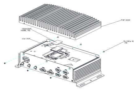
**Step 3**: Gently place the CPU into the socket without applying force, then close the socket cover and secure the metal retention arm. Prior to reassembling the chassis, ensure a thermal pad is affixed on top of the CPU.
