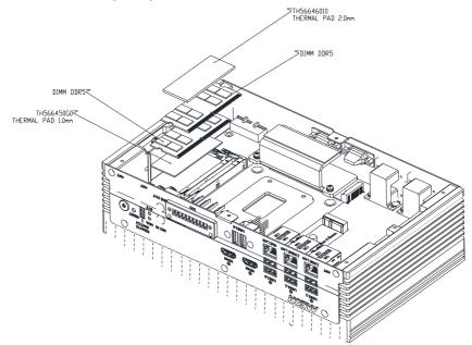
**Step 1**: If not already disassembled, remove the eight (8) screws from the bottom cover of the system, as located in the below diagram (circled).
