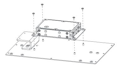
**Step 4**: Secure the bracket using four (4) screws through the base of the bracket into the standoffs on the chassis.
