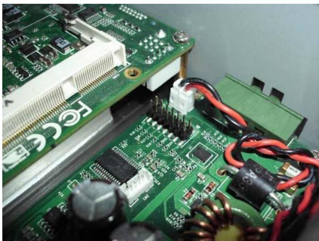
For +24V DC input, a jumper is needed
