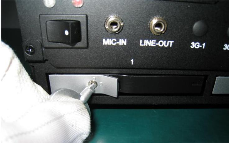
2. Slot in the storage device (For removal, the storage device will be mechanically pushed out when the bay door opens)
