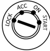
Since voltage requirement for ACC is usually the same as voltage of the battery, users may connect V+ with ACC to power up BOXER-6301VS. See the picture below.
