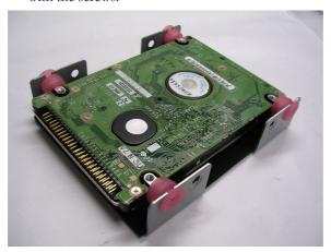
**Step 5:** Cover it with another piece of iron surface and lock it with the screws.
