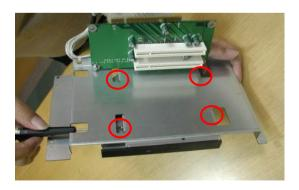
Step 3: Push the CD-ROM module into the board.
