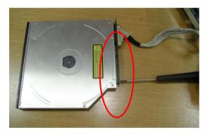
**Step 2:** Fix the CD-ROM on the iron bracket with screws.
