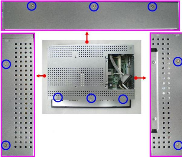
Step 2: Take off the back cover of AOP-8120XT and change the jumper setting
