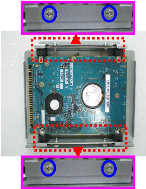
Step 3: Plug IDE cable to the HDD with HDD kit and then fasten the HDD kit on the back cover of the AOP-8120XT with four screws
