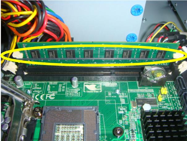
Step 2: Put a rubber band around the RAM to secure it in the slot
