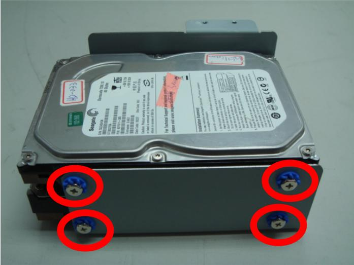
Step 4: Put the HDD back to the chassis by sliding HDD and lock to the position.
