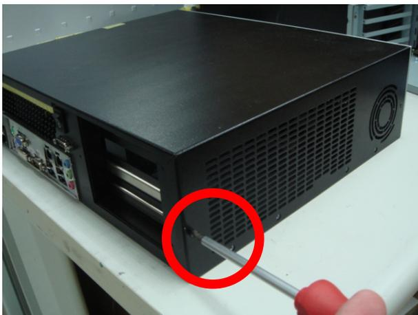
Step 2: Unfasten the screws of the HDD bracket and pull out the bracket
