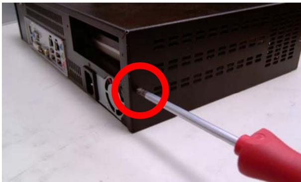
Step 2: Unfasten the two screws on the two sides of the HDD bracket
