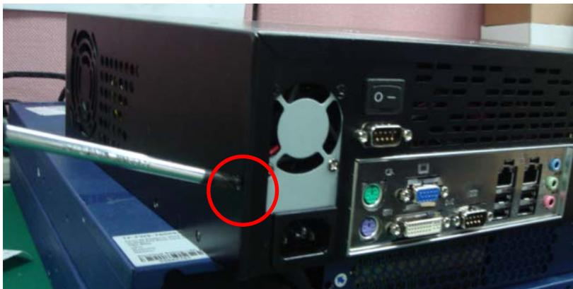
Step 2: Unfasten the screw of the HDD bracket and pull out the bracket
