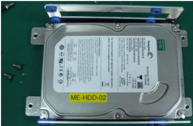
Step 4: Fasten the two screws on the HDD bracket
