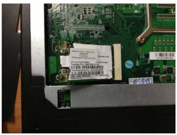
Step 4: Fasten the two M2.5 screws on the Mini PCIe Card
