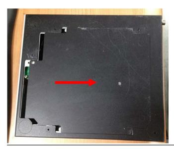
Step 3: Insert the CFast Card to the CFast slot and finish installation
