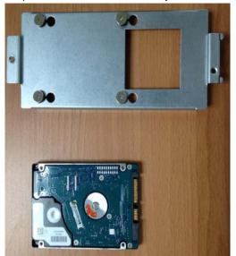
Step 6: Put the HDD to the HDD bracket and fasten the four screws
