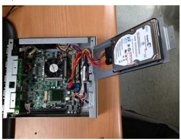
Step 8: Close the HDD bracket and finish the installation
