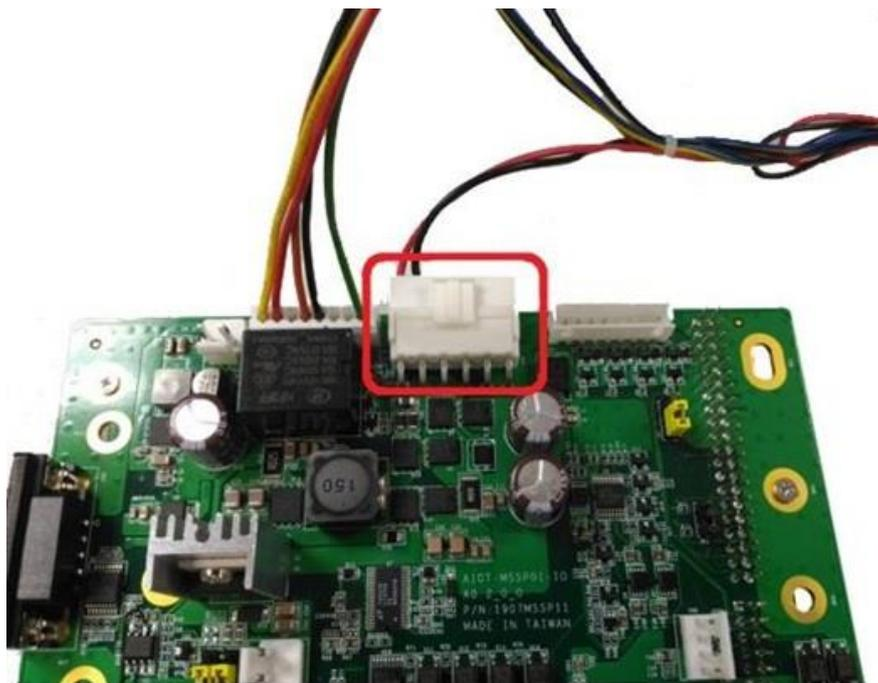
**Step 11:** Plug the barrel plug of the 24V power supply to the barrel end of the 24V power cable that's connected to the AAEON computing board.
