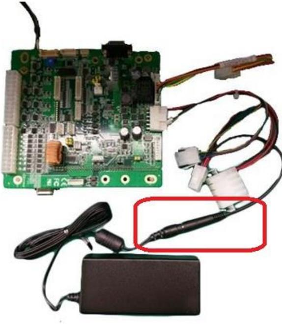
**Step 12:** Plug the AC power cord in to the 24V DC power supply's receptacle. Now plug the 24V DC power supply's AC cord plug in to an 110V AC outlet.
