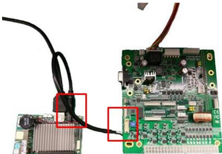
**Step 10:** Plug the 6-pin in-line end of the 24V DC input power cable in to the CN4 connector on the AAEON vending I/O board.
