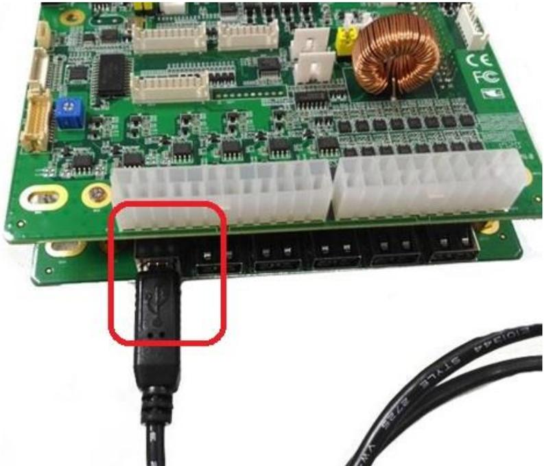
**Step 3:** Plug the type A end of the included USB cable in to one of the USB type A connectors (any USB connector is fine) on the AAION computing board.
