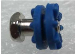
Step 4: Get the screws from the rubbers and insert the anti-vibration rubbers into the fillister of the HDD bracket first
