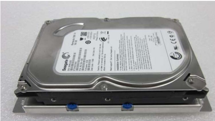
**Step 7:** Connect the SATA and Power Cables to the HDD
