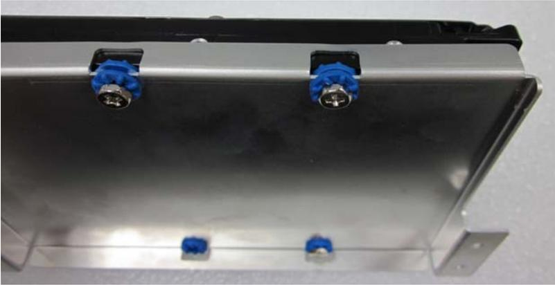
Step 6: Put the HDD to the HDD bracket
