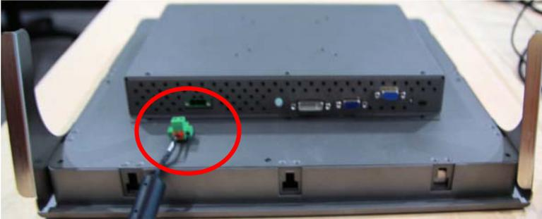
A "Surge Protection" device plugged between the AC-DC adapter and the wall outlet is recommended to prevent the effects of sudden current variations from reaching the LCD Display. The sudden peaks of electricity may harm the LCD Display.
