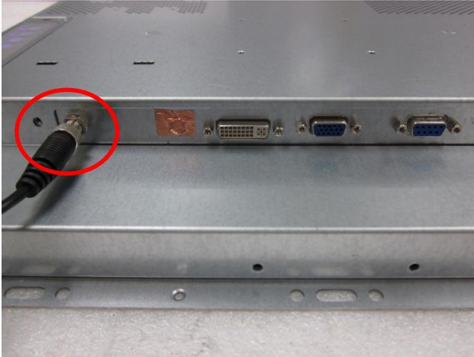
A “Surge Protection” device plugged between the AC-DC adapter and the wall outlet is recommended to prevent the effects of sudden current variations from reaching the LCD monitor. The sudden peaks of electricity may harm the LCD monitor.
