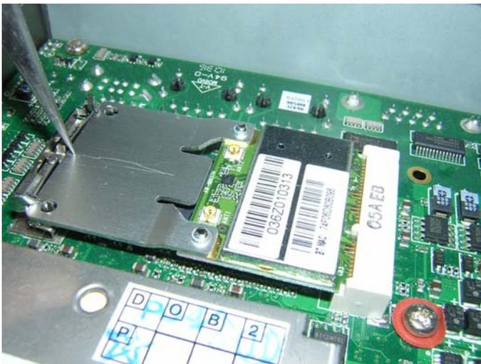
Step 2: Connect the antenna cable to the connector on WiFi Card
