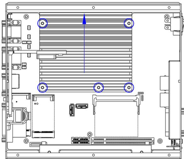
Step 11: Fasten the six screws on the bottom lid.
