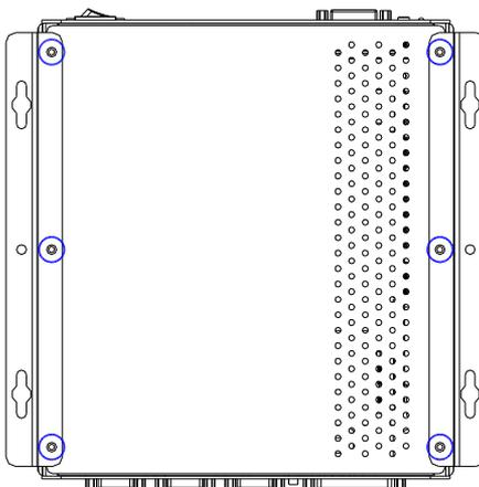
Step 3: Unfasten the five screws on the heatsink and remove the heatsink
