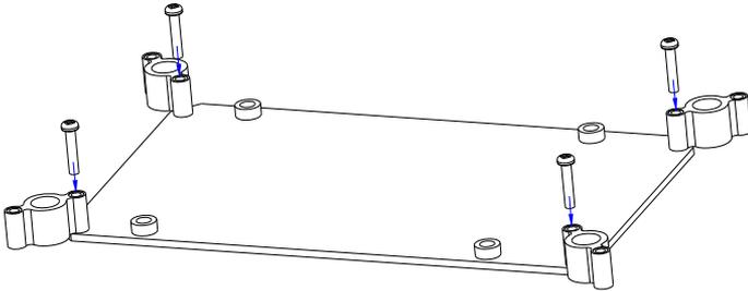
Step 4: Fasten the four screws to fix the HDD with the HDD bracket
