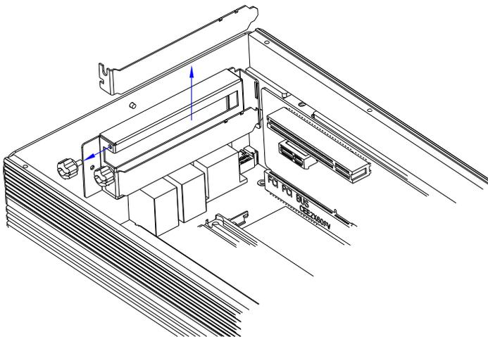
Step 4: Insert the PCI/PCI-Express card into the PCI/PCI-Express slot and reattach the screw.
