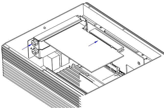
Step 5: Unfasten the screws and push the tenon to lock the PCI/PCI-Express card in position
