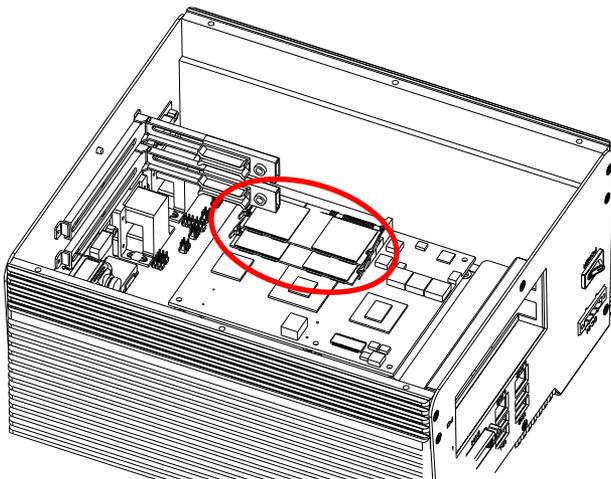
Step 10: Place the heatsink on the memory and push the heatsink against the chassis, and then fasten the five screws
