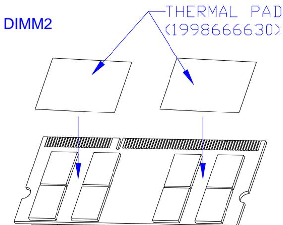
Step 9: Install the DIMM2 to the upper layer of the memory slot
