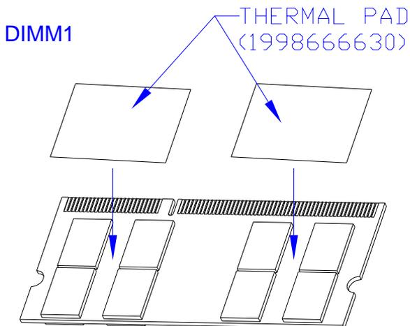
Step 6: Install the DIMM1 to the lower layer of the memory slot
