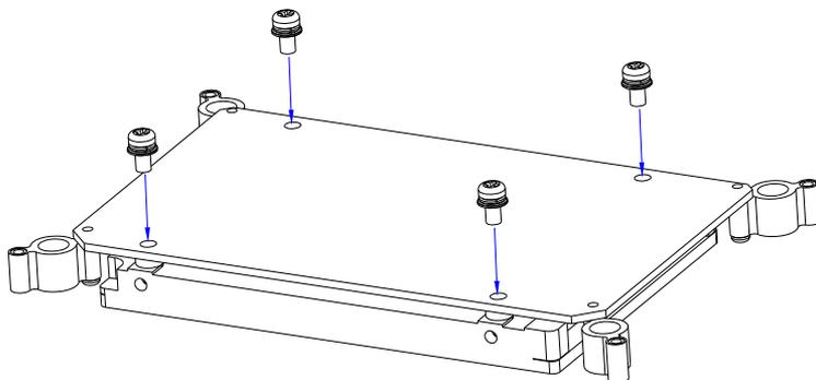
Step 5: Fasten the four screws to fix the HDD bracket with the AEC-6924 chassis
