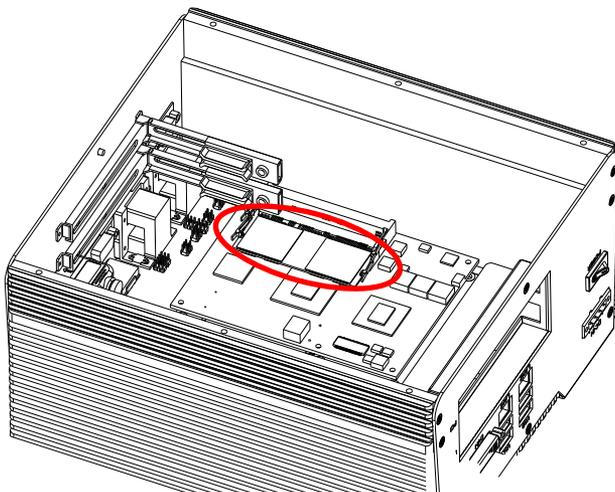
Step 7: Adhere the two thermal pads (1998666630) to the diode of facade of memory DIMM 2
