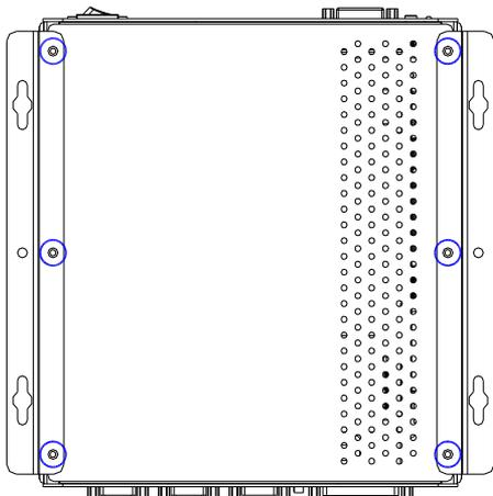
Step 12: Fasten the screws on the rear panel and front panel
