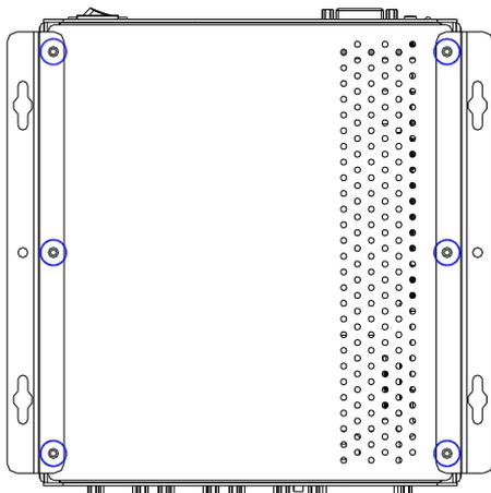
Step 7: Fasten the screws on the rear panel and front panel
