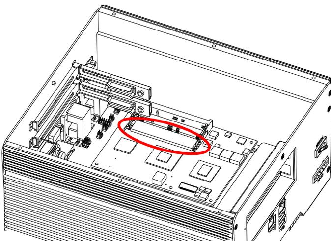
Step 5: Adhere the two thermal pads (1998666630) to the diode of facade of memory DIMM 1
