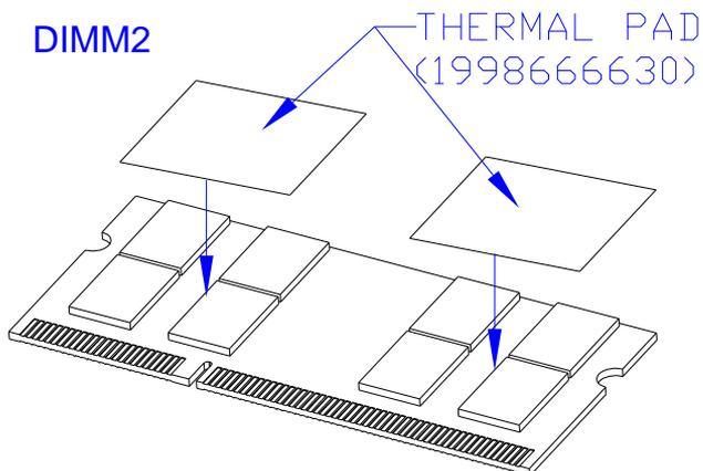
Step 8: Adhere the two thermal pads (1998666630) to the diode of other side of memory DIMM 2
