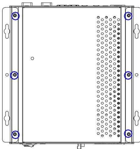
**Step 8:** Fasten the one screw on the rear panel and one screw on the front panel
