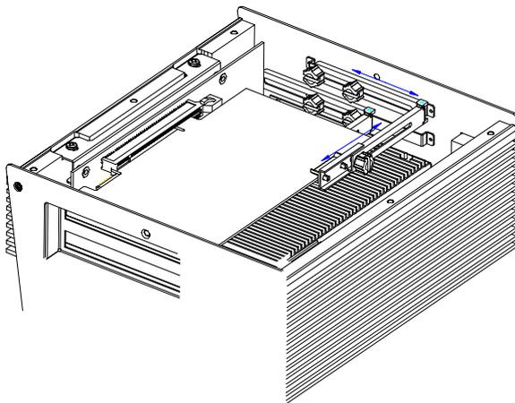
Step 7: Close the bottom lid of the AEC-6911 and fasten six screws on bottom lid.
