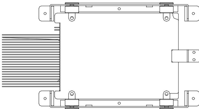
Connect the HDD cable (for SATA Type HDD)
