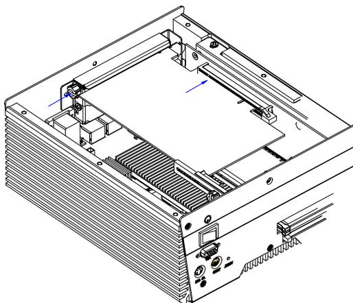
Step 6: Unfasten the screws and push the tenon to lock the PCI card in position.
