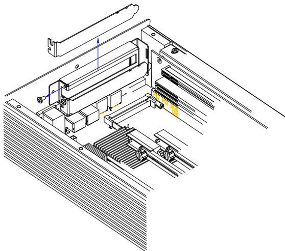
Step 5: Insert the PCI card into the PCI slot and reattach the screw.
