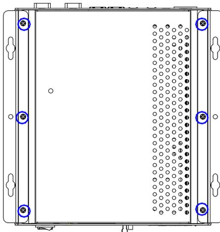
Step 4: Remove the screw with your finger and get the PCI card ready to install. You should keep the shield and screw for use later.
