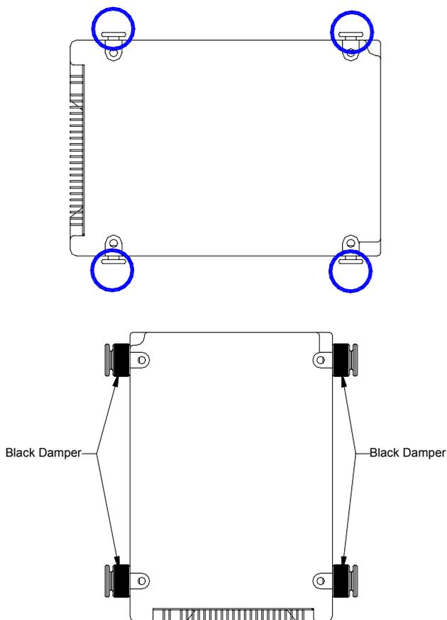
**Step 2:** Assembly the HDD chassis
