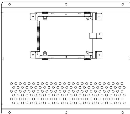
**Step 3:** Assembly the damper bracket
