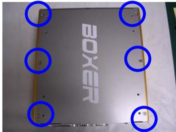
**Step 4:** Remove the screw with your finger (figure 1) and get the PCI card ready to install. You should keep the shield and screw for use later.
