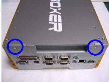
Step 2: Unfasten three screws on the front panel.
