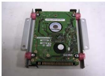
Step 3: Connect the power cable to the HDD module. (Red wire is Pin 1)
