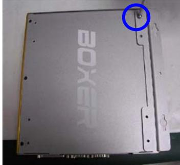
Step 2: After fastening the two brackets on the bottom lid of AEC-6900, the wallmount kit installation is finished.
