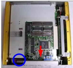
**Step 6:** Unfasten the screws (Figure 1) and push the tenon to lock the PCI card in position (Figure 2).
