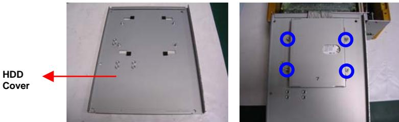
Step 5: Close the HDD cover and fasten the five screws on the HDD cover. Close the bottom lid of the AEC-6900 and fasten six screws on the bottom lid; the HDD installation is now finished.
