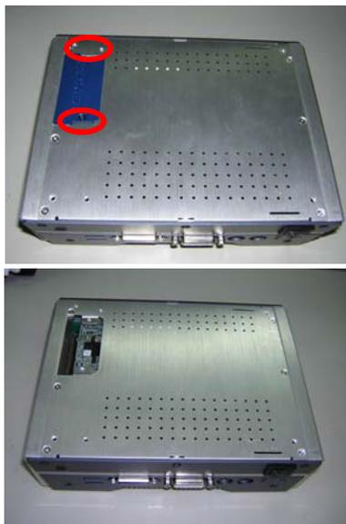
Step 2: Insert the other side of HDD cable and power cable into the slots on the bottom of the chassis.
