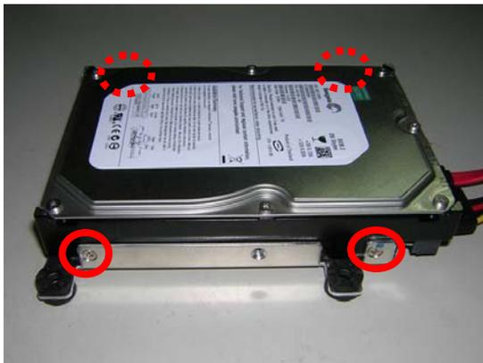
Step 5: Get the screws ready, by matching them up with a washer. Meanwhile, place the HDD kit into the HDD kit housing and then screw the HDD kit to the HDD kit housing.
