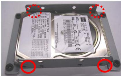
Step 3: Fasten the second HDD module to the bracket with screws.
