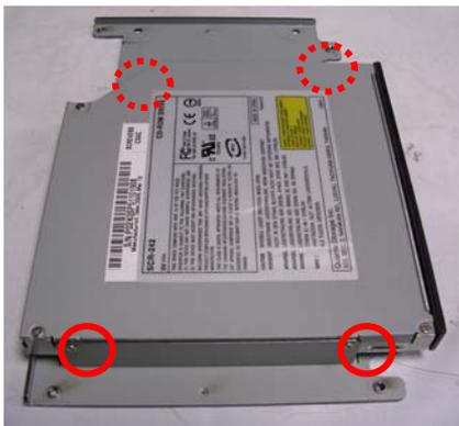
Step 3: Fasten the Riser Card and the CD-ROM with screws.
