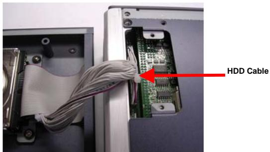
Step 3: Combine the chassis with the HDD kit housing and then lock with screws.
