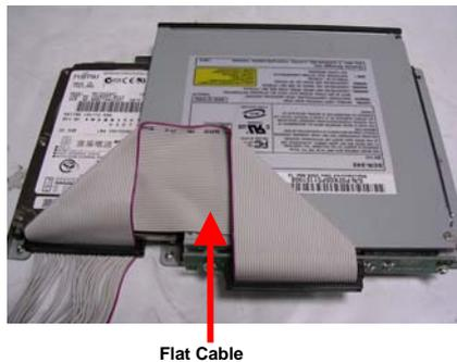
Step 6: Place the CD-ROM and HDD kit into the suitable plate and then reverse it. Screw the CD-ROM and HDD kit to the plate.
