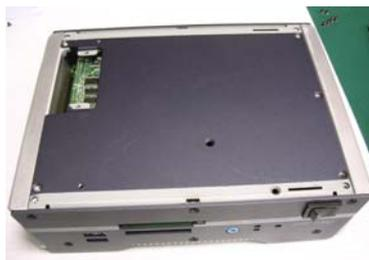
Step 2: Insert the other side of flat cable into the slot on the bottom of the chassis.
