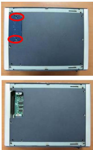
Step 2: Insert the other side of HDD cable and power cable into the slots on the bottom of the chassis.
