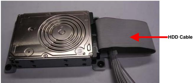
Step 5: Place the HDD kit into the HDD kit housing and then screw the HDD kit onto the HDD kit housing.
