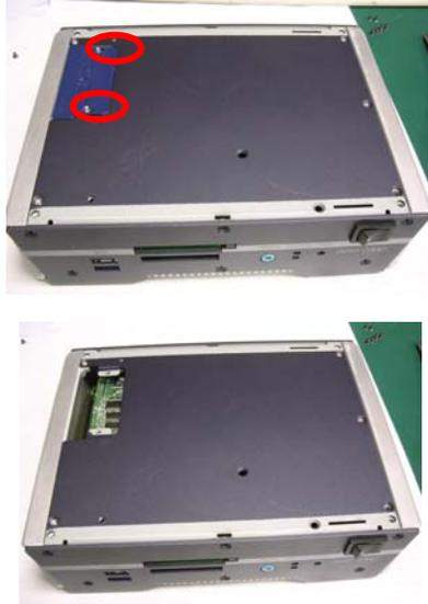
Step 2: Insert the other side of HDD cable into the slot on the bottom of the chassis.
