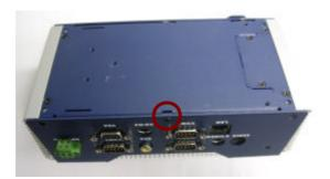
**Step 2:** Remove the lid after you screw the lid off the chassis and insert the DDR SDRAM SODIMM module into the slot.
