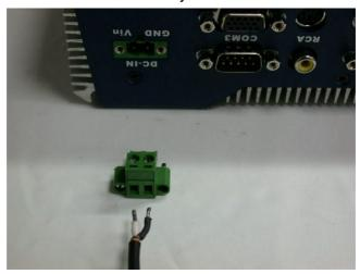
Step2: Fix the connector to the cable with the screws.
