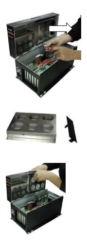
• Unscrew the mounting bracket from the chassis.
