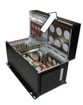
• Unscrew the cover, lift the lid and keep the top of the chassis open.
