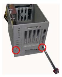
Step 4: Separate the bottom cover from the chassis
