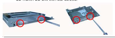
Step 4: Replace the whole unit back to the Chassis
