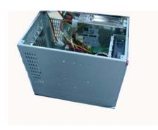
Note: Don't forget to attach the face plate to the opening slot in the front of the chassis
