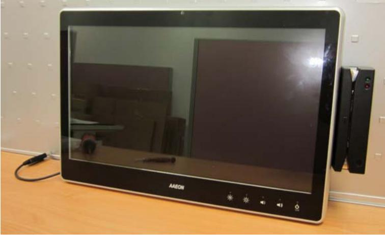
Step 1: Fasten the two screws (2-SELF TAPPING SCREWS) to fix the MSR Bracket with the ACP-5215
