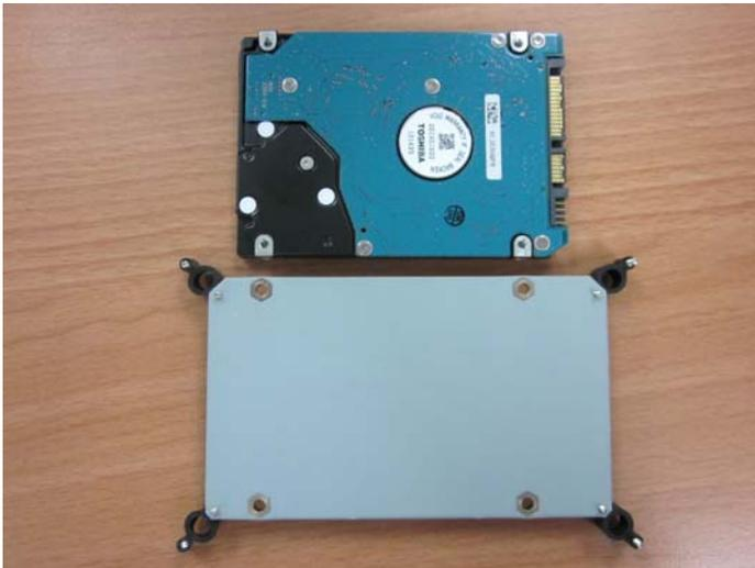
Step 5: Fasten the four screws to fix HDD Bracket and HDD
