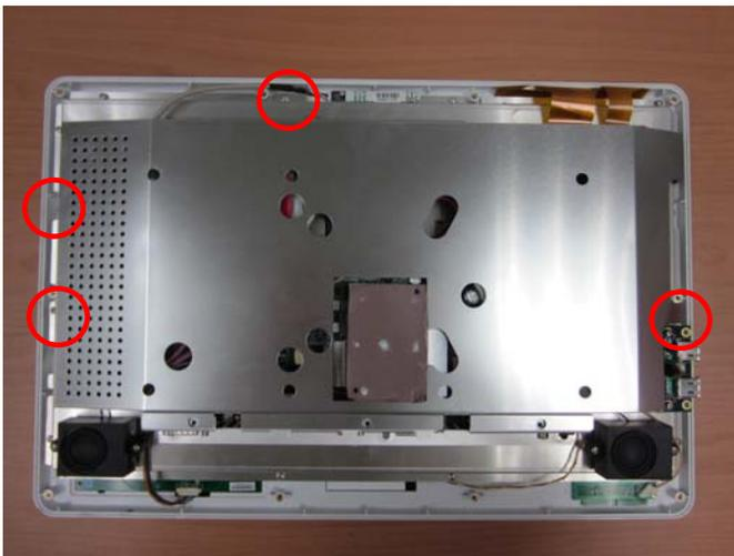
Step 3: Remove HDD Bracket (4 screws)
