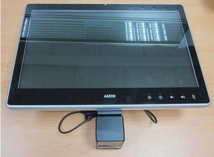
Step 1: Fasten the three screws to fix the Bar Code Scanner with the bracket
