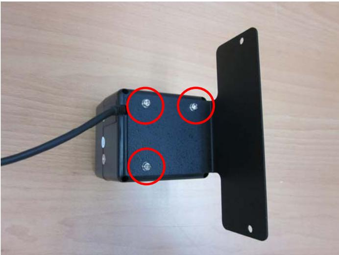
Step 2: Fasten the two screws (2-SELF TAPPING SCREWS) to fix the Bar Code Scanner with the ACP-5215
