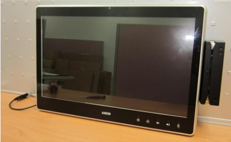
Step 1: Fasten the two screws (2-SELF TAPPING SCREWS) to fix the MSR Bracket with the ACP-5210
