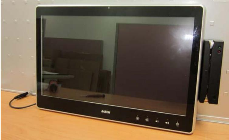
Step 1: Fasten the two screws (2-SELF TAPPING SCREWS) to fix the MSR Bracket with the ACP-5185
