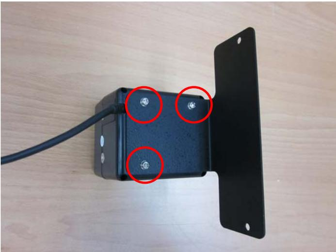
Step 2: Fasten the two screws (2-SELF TAPPING SCREWS) to fix the Bar Code Scanner with the ACP-5185
