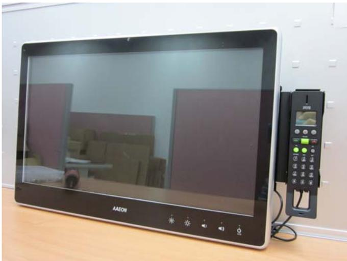
Step 1: Fasten the two screws(2-SELF TAPPING SCREWS) to fix the Skype Bracket with the ACP-5185
