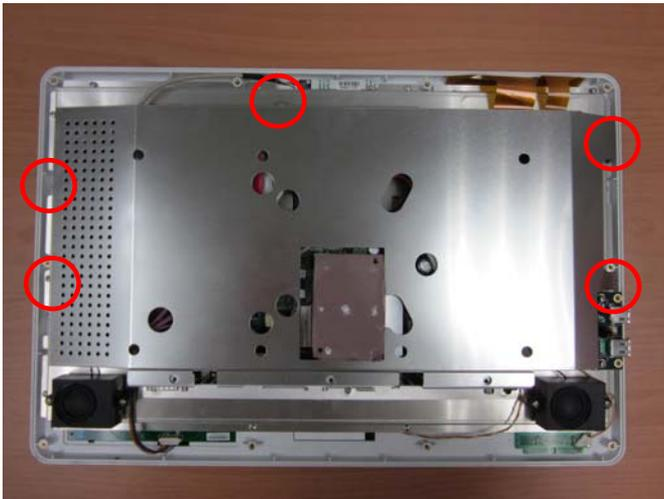
Step 3: Remove HDD Bracket (4 screws)
