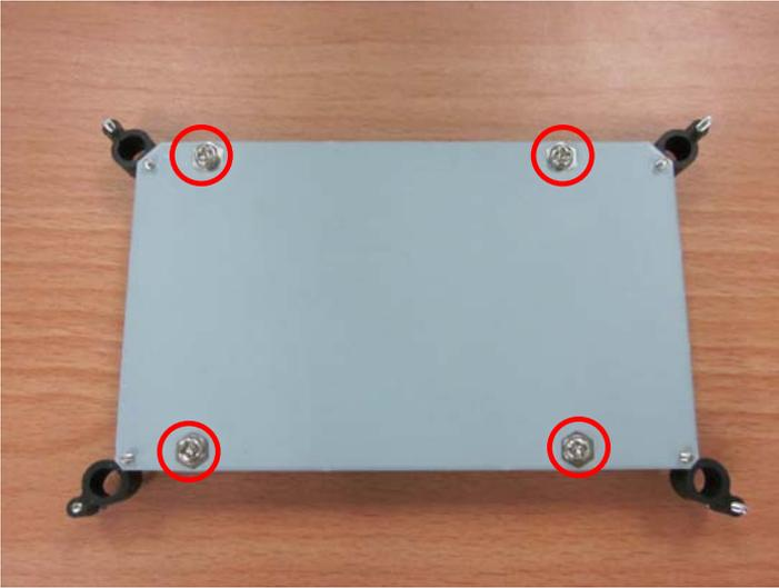
Step 6: Connect the SATA and power cables to the HDD and fasten the four screws to fix the HDD Bracket
