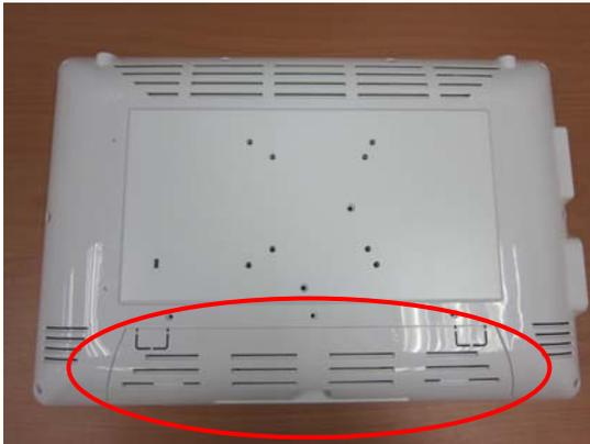
**Note 1:** You may turn on the power by cutting and destroying the protective cover as it shows below.
