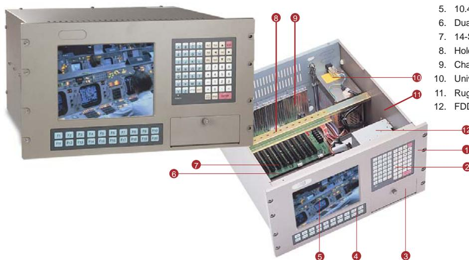
1. 19" aluminum sealed alloy front panel
