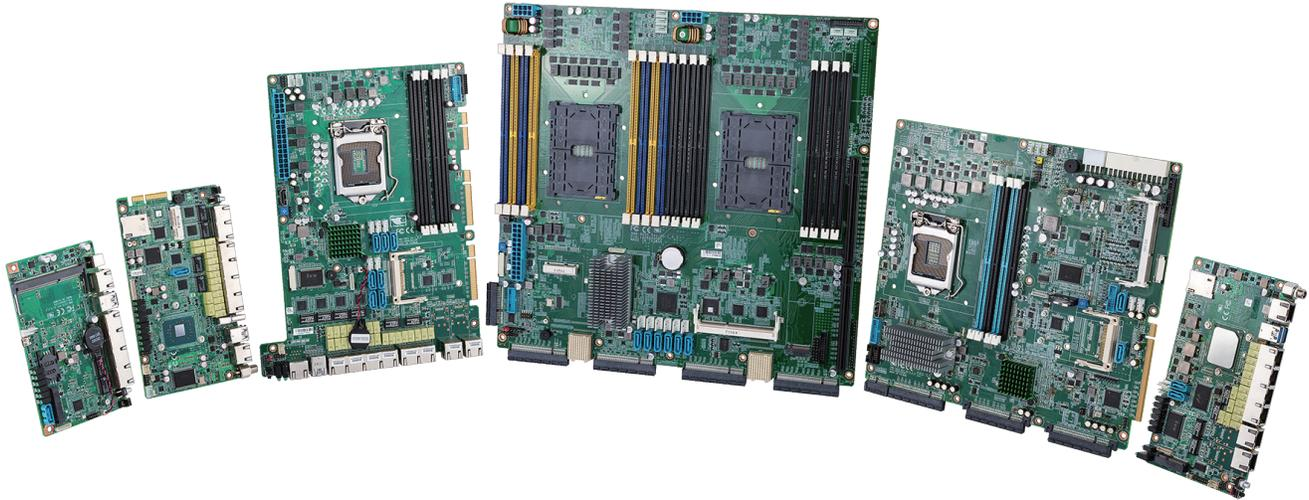
AAEON provides a wide range of network motherboards based on the Intel® X86 platform and built with the latest generation Intel® CPU and high performance LAN chip from Intel® Atom™ all the way to Intel® Xeon processors. All AAEON network motherboards feature GbE, advanced LAN bypass functions, wireless connectivity via Mini-PCIe slot or M.2 interface, RJ-45 consoles, and high speed USB functions.
