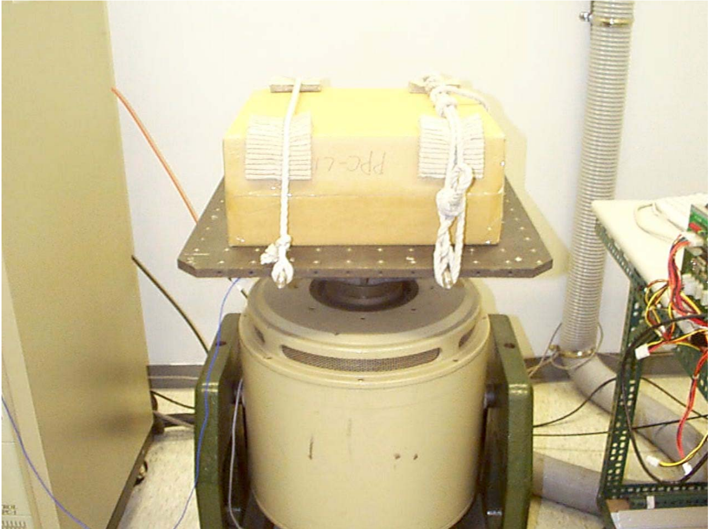
PC3-P200 package vibration test for Y-axis
