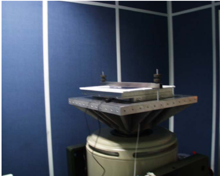
AMB-280A operation random vibration test for Z-axis
