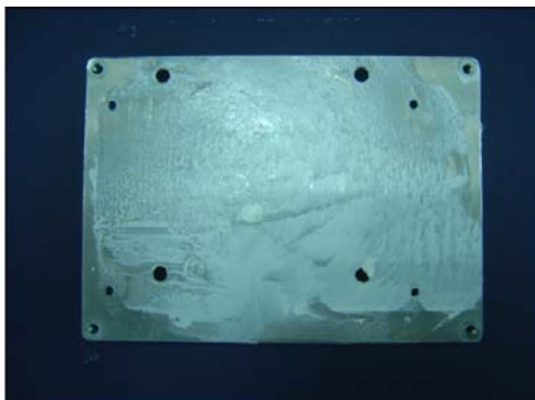
Heat-Spreader (P/N: M10BT01010) + Thermal Pad
