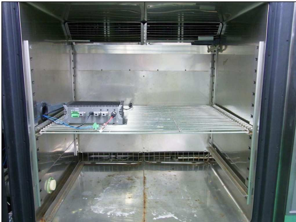
Figure 11 : Damp Heat Test, Cyclic Setup
