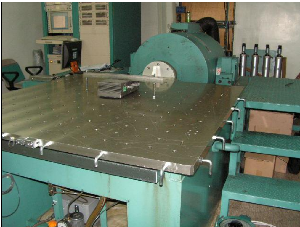
Figure 38 : Mechanical shock test for longitudinal axis
