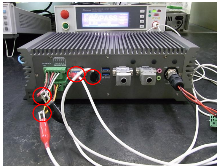
Figure 44 : Dielectric withstanding voltage test
