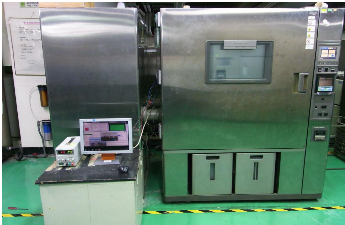
Figure 6 : Dry heat and extra over-temperature test
