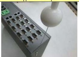
Test for protection against access to hazardous parts and against solid foreign objects
