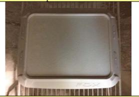
Test for protection against solid foreign 6. objects (Dust test)
