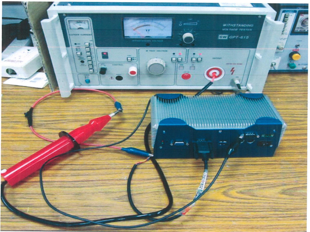
Dielectric Strength Test
