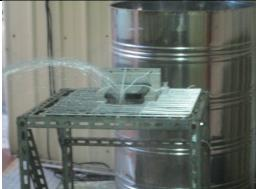
Test for protection against water (Bottom)
