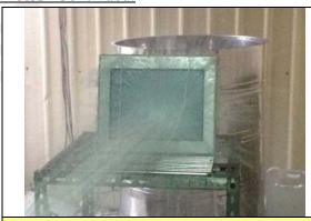
Test for protection against water (Front face)
