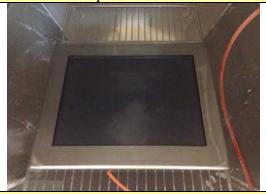
Test for protection against solid foreign objects (Dust test)
