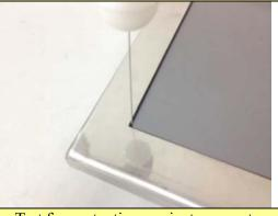
Test for protection against access to hazardous parts
