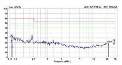
Condition: limit\FCC\FCC Part15B CLASS-A QP.csv Line
