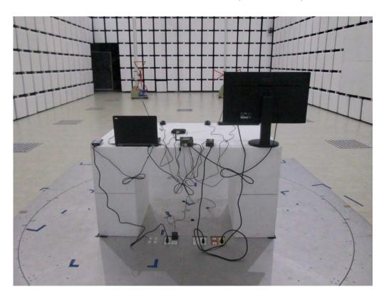
**Radiated Emission - Front View (Above 1GHz)**
