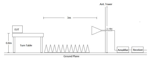
The radiated disturbances below 1GHz tests were performed in the 3 or 10 meters Chamber test site, above 1GHz tests were performed in the 3 meters Chamber test site, using the setup accordance with the ANSI C63.4-2014. The specification used was the FCC Part 15.109 Class A limits.
