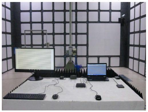
Radiated Emission - Rear View (Above 1GHz)
