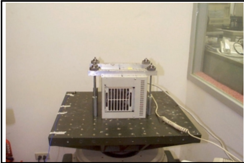
X-Axis 1G random vibration test
