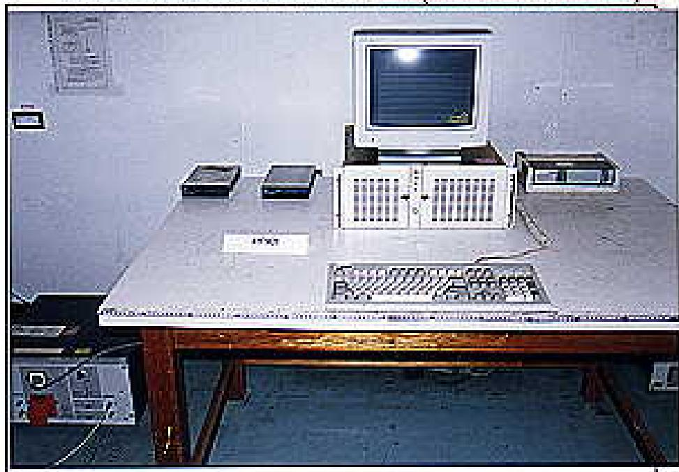
CONDUCTED EMISSION TEST (MODEL: SBC-490)
