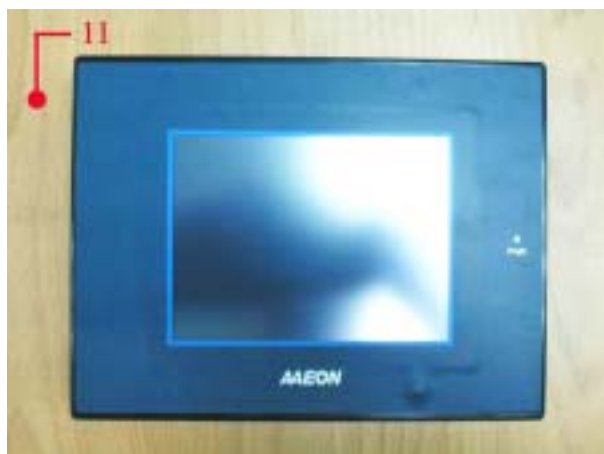
AOP-8060 (MPC-5320 A1.0) Fanless Operator Panel PC
