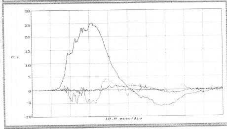
DROP TEST NAME Mica-151 DROP TEST ITEN 1.3.6 92CM DROP TEST FACE RIGHT DROP TEST P.S CHANNEL 2
