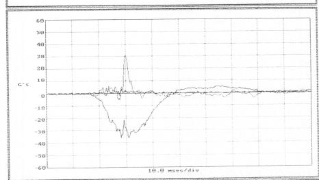
DROP TEST NAME Mica-151 DROP TEST ITEN 1.3.6 92CH DROP TEST FACE BOTTOM DROP TEST P.S CHANNEL 1 NOTES:
