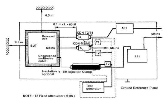
*Note:* 1. *The EUT is setup 0.1m above Ground Reference Plane* 2. *The CDNs and / or EM clamp used for real test depends on ports and cables configuration of EUT.*
