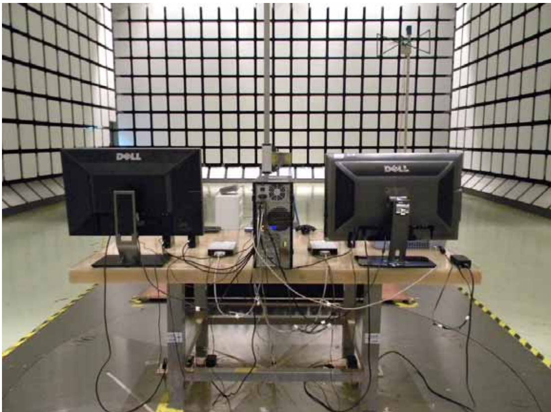
Back View of Radiated Measurement
