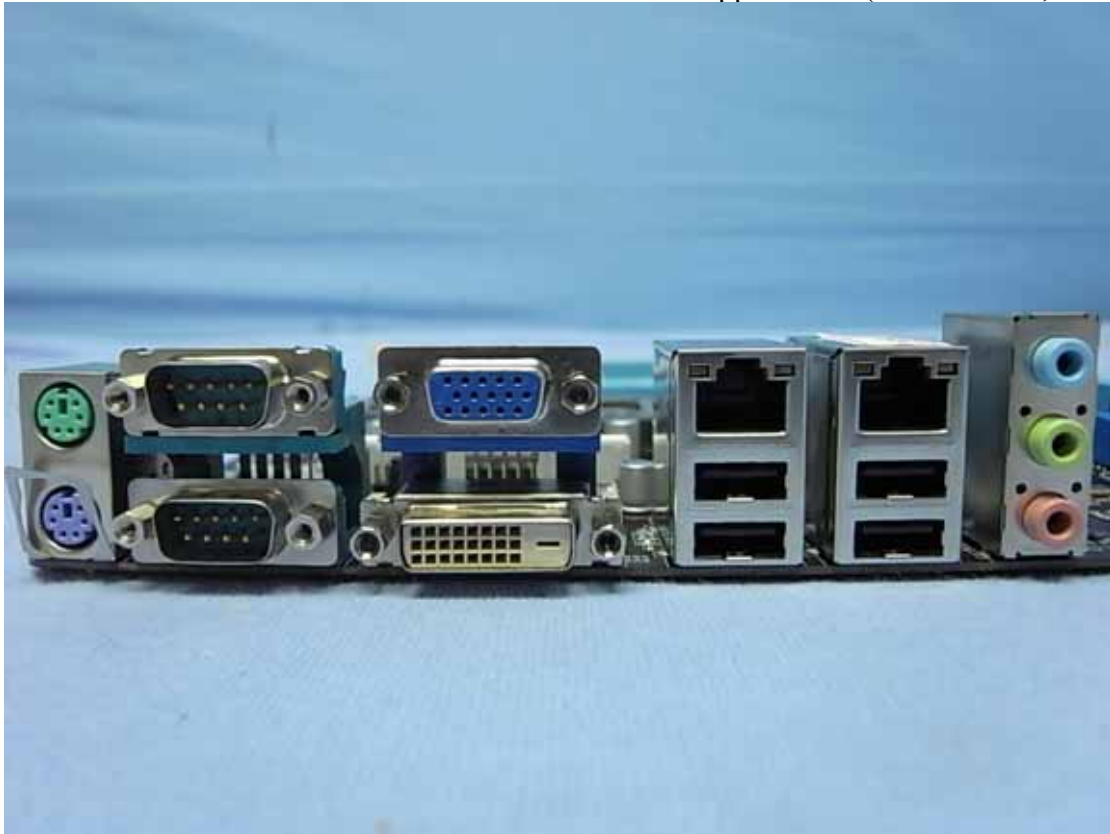
Figure 5 General Appearance (Motherboard, I/O Ports)
