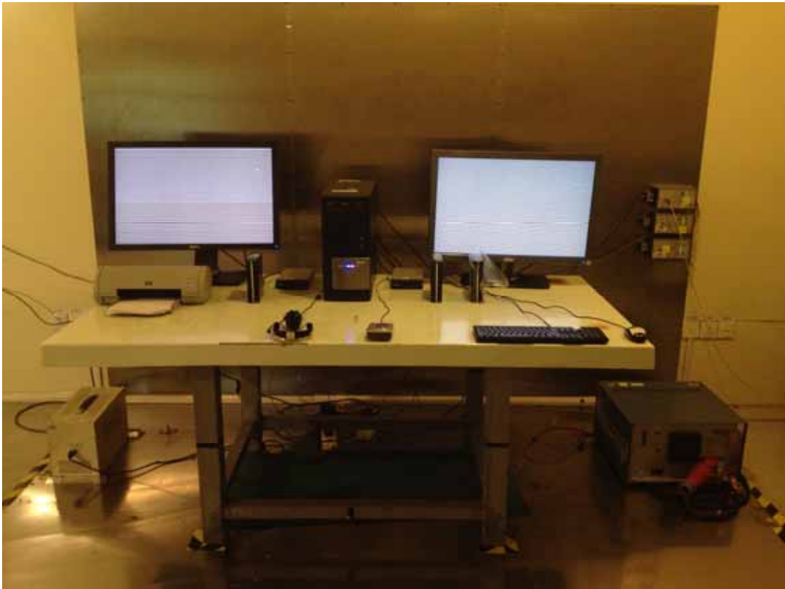
Front View of Conducted Emission Measurement (Telecommunication port)
