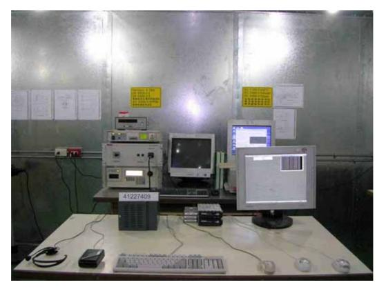
CONDUCTED DISTURBANCE, INDUCED BY RADIO-FREQUENCY FIELDS TEST
