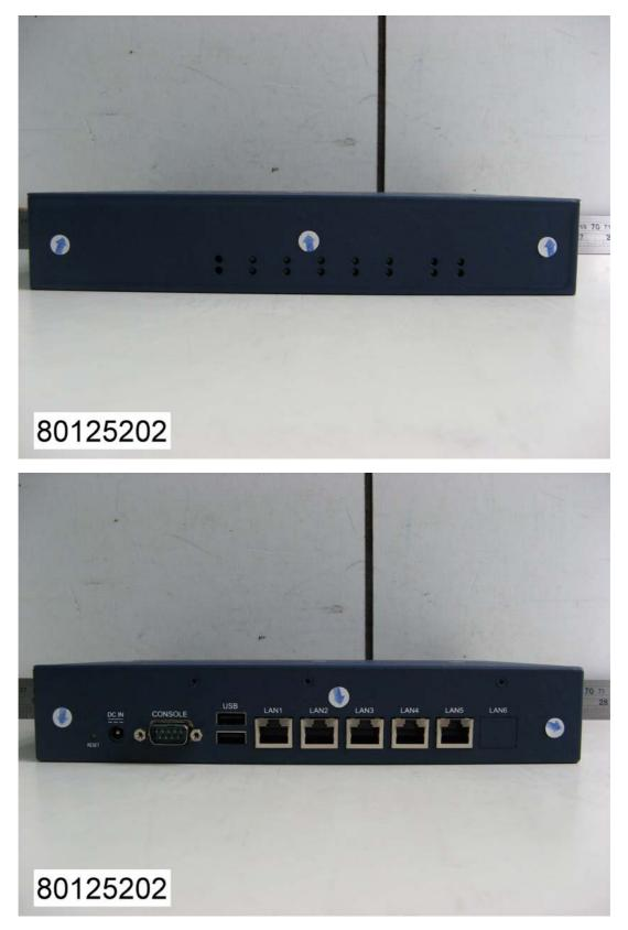
Red Dot —Air Discharged Blue Dot —Contact Discharged
