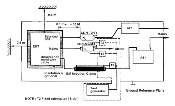
Note: 1. The EUT is setup 0.1m above Ground Reference Plane
